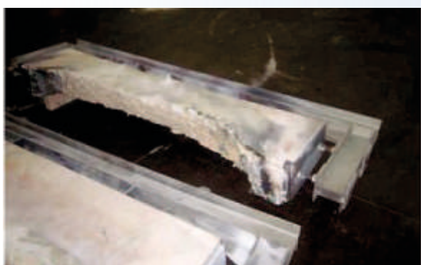
◆ Dog house arch in one piece zircon-mullite after 7 years
